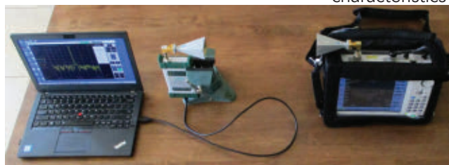
▲ Fig. 4 Link measurement setup at 28 GHz. A 0 dBm, battery-powered portable source drives the transmit antenna, with a handheld spectrum analyzer connected directly to the receiving antenna.
