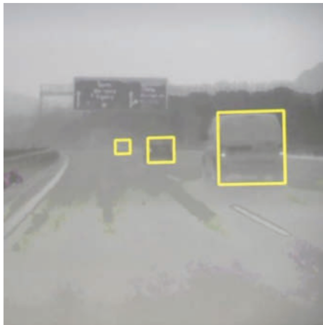
▲ Fig. 2 Millimeter wave radar has the ability to penetrate dust and fog, which enables it to accurately detect and identify other vehicles and road hazards.
