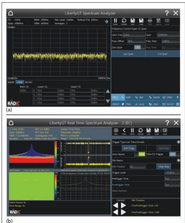
▲ Fig. 1 A 300 ns pulse eludes detection in a typical spectrum analyzer (a) yet is readily detected by the LGT1410 RTSA (b).
